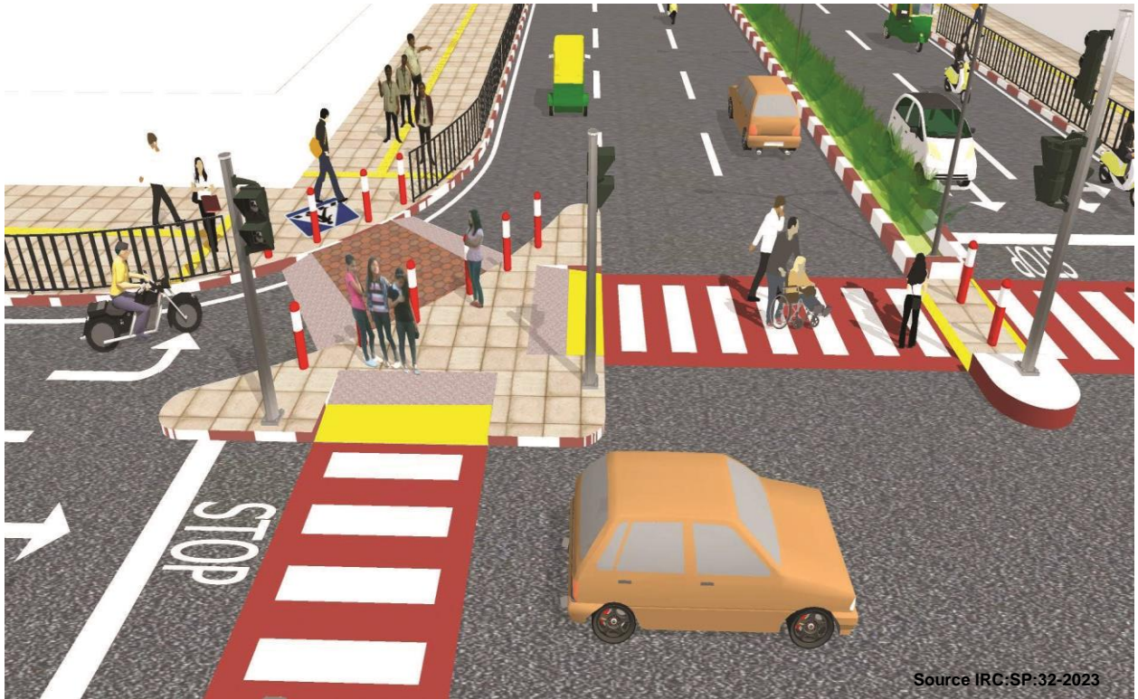
Figure 18 Refuge Island with safe gap for pedestrians
