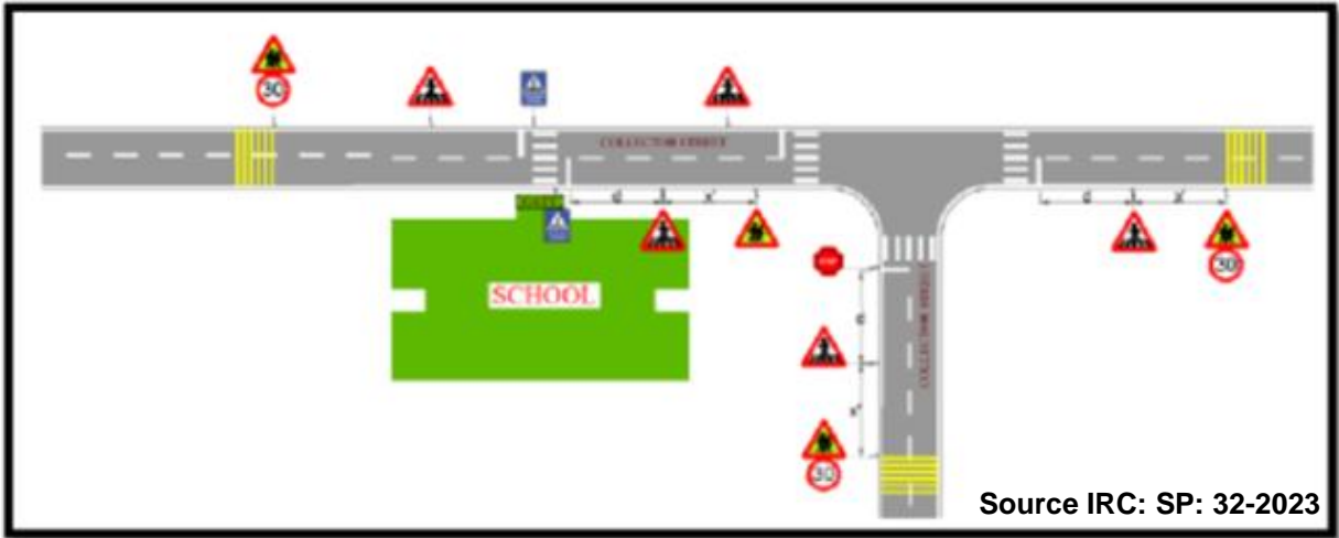
Figure 4 Typical illustration of various measures required for the School Gate located on the Midblock Location of Two-Lane Bidirectional Road
